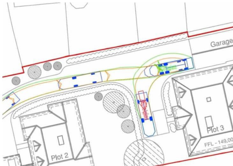
Swept Path Analysis example, Image provided by Lapworth Architects
