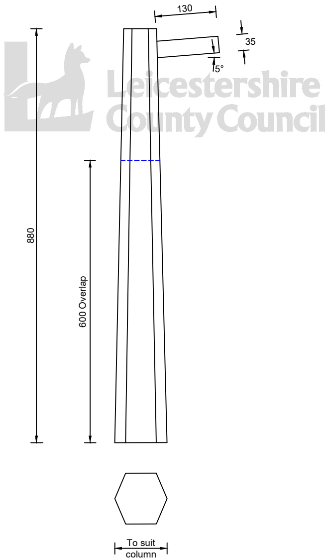
TYPICAL SLEEVE BRACKETS FOR 5/6m COLUMNS
